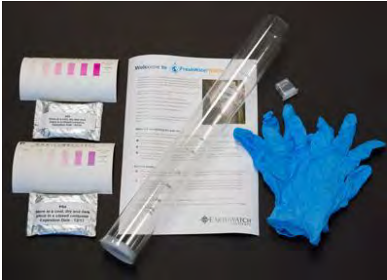
Figure 4 FreshWater Watch kit that includes method for determining nutrient pollution (nitrate and phosphate), particulate (sediment) concentrations and algal blooms
